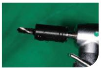
• Ø2.8 → Ø3.1 CAS-Drill (800 rpm) A 5 mm Stopper is used for the final drilling and lifting of the membrane.
