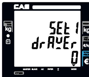
② Press appropriate numeric key to set pulse length of 1~99 (ms) and
